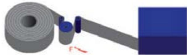
Film trolley with electromagnetic brake. This can be adjusted from the control panel.
